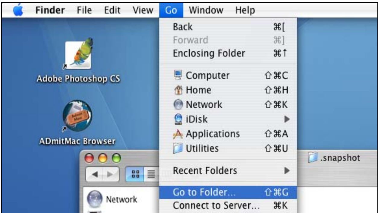
Figure 17) To restore from a Snapshot copy using Finder on NFS mounts, use “Go to Folder”...
